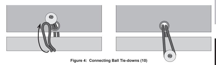
4. Use the Ball Tie-downs (10) to attach the Roof Tarp to the tubes using the eyelets on the eyelet straps.
